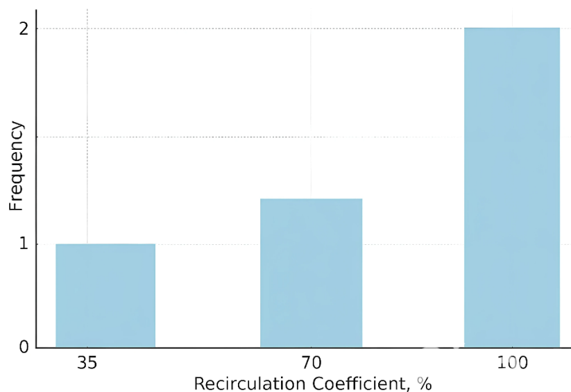
Figure 3. Distribution of water recirculation ratios across different system scales, campus-level installations achieved 100% recycling, while large municipal plants averaged 33% due to regulatory discharge constraints
