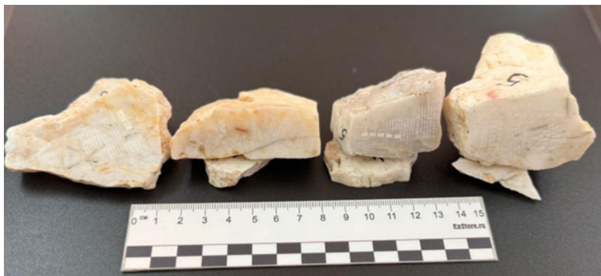
Figure 2. Quartz specimen with LIBS impact-points
