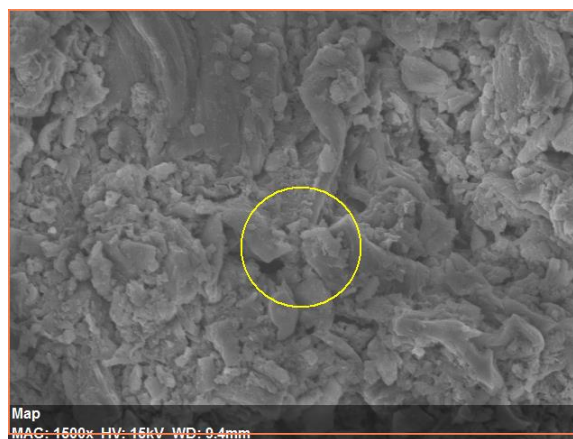
Figure 3. SEM images of pine cone-based activated carbon
