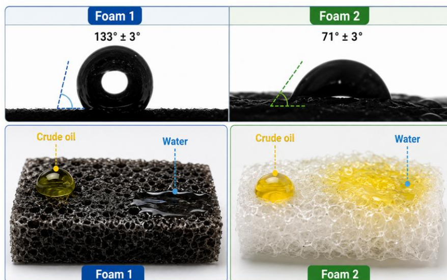
Figure 7. Wettability of foams by water and crude oil. Water and crude oil were colored for better visibility (derived from Hailan et al., 2025)
